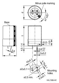
Snap-in capacitors are also available with 3 terminals (length (4.5-1.4) mm). PET insulation cap is positioned under the insulation sleeve. Safety vent on the base.
