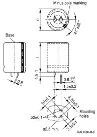
Snap-in capacitors are also available with 3 terminals (length (4.5 -1) mm). PET insulation is marked with label "PET" on the sleeve. Safety vent on the base.
