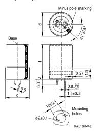
Snap-in terminals, length (6.3 + 1/-1.4) mm. Also available in a shorter version with a length of (4.5 - 1.4) mm. PET insulation cap is positioned under the insulation sleeve. Safety vent on the base.
